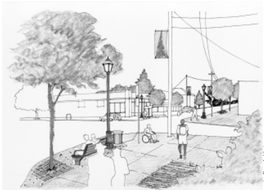
Curb extensions at transit stops would provide room for new lighting, benches or shelters, trash cans and street trees.
