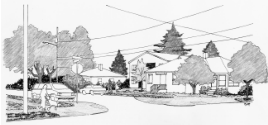
Curb extensions at the entries of selected residential streets will help slow traffic entering these streets.
