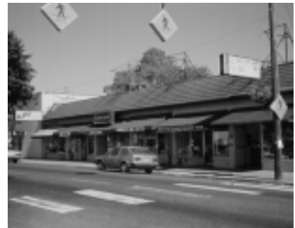
Overhead pedestrian crossing signs can be used to improve the visibility of pedestrian crossings.
