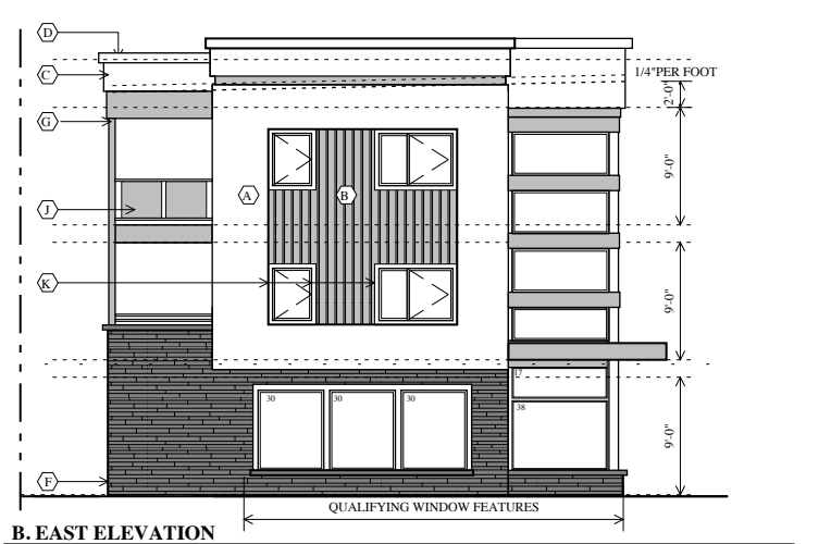
B. EAST ELEVATION 1/8" = 1'-0" 40% WINDOW COVERAGE @ GROUND FLOOR PLANNING AND ZONING: WALL AREA BETWEEN 28'-0" ABOVE GRADE = 319 SF * 40% = 127.6 SF MIN. PROVIDED: 145 SF
